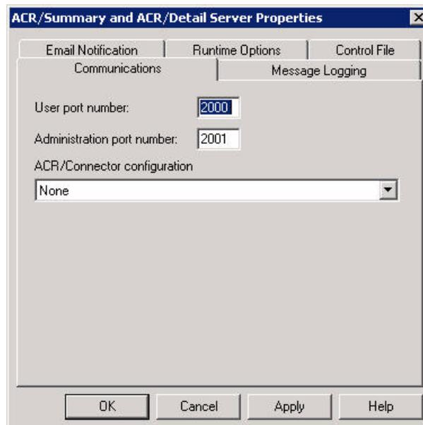
The **User port number** and **Administration port number** display the Communication Parameters established during installation, as described in [step 5 on page 9](#). The above example shows the default port
